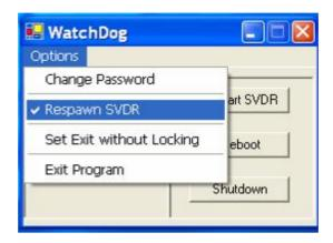
The Super User can prohibit the WatchDog from constantly restarting the critical applications by unselecting the **Respawn S-VDR** label. When exiting, the WatchDog automatically locks the Task Manager. To prohibit that select the **Set Exit Without Locking** label.
